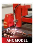
The Machine equipped with smart height controller for effectively cutting. The Plate ranging from 3 mm to 38mm thickness using air plasma
